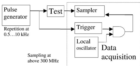
Fig. 4. Generic architecture of the first data acquisition system: the pulse generator and local oscillator are independent.
