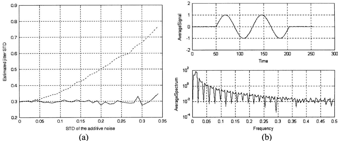
Fig. 2. (a) Simulation of the noise immunity of the two algorithms (true value of the frame jitter STD is 0.3, solid line—first algorithm, dashed line—second algorithm). (b) Test signal and its spectrum.
