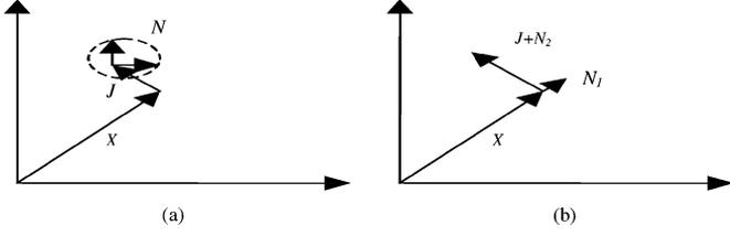
Fig. 1. Phasor diagrams of the recorded spectra ( $X$ —true signal,  $N$ —additive noise,  $J$ —frame jitter), (a) before and (b) after rotation of the additive noise components.
