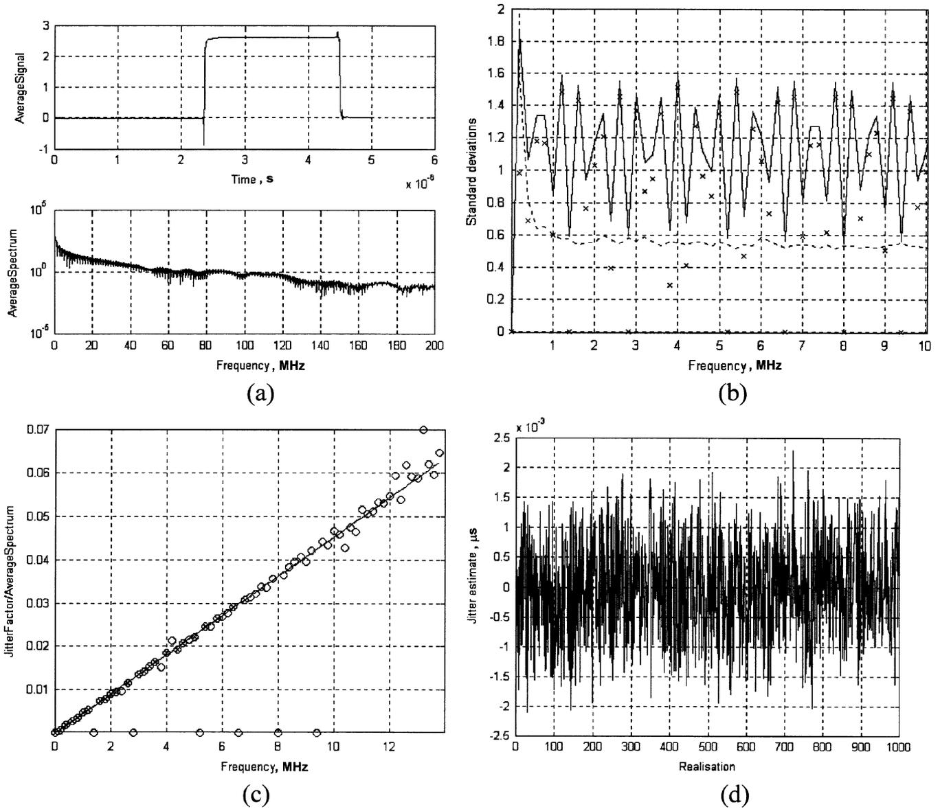
Fig. 3. Application of the algorithms to the experimental analysis of a rectangular pulse. (a) Averaged pulse and the averaged spectrum. (b) Standard deviations of the spectrum components (solid line—quadrature, dashed—in-phase), and their difference (crosses). (c) Jitter factor—experimental points and regression line. (d) Estimated time shifts.
