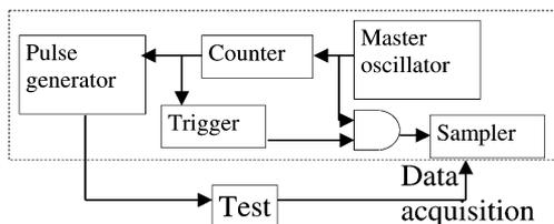
Fig. 6. Generic architecture of the second data acquisition system: the pulse generator is triggered by the master clock.
