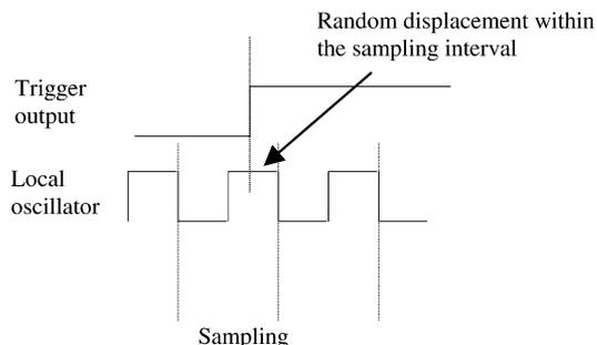
Fig. 5. Appearance of the random time shift between the trigger event and start of sampling that is evenly distributed within the sampling interval.
