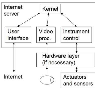
Fig.1. Remote laboratory based on a software server
